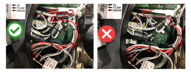
LN-25X: Lead 707 being rerouted thru toroid. Direction arrows show routing from flexible power pc board to user interface pc board.
