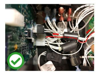
Activ8X: Lead 707 being rerouted thru toroid. Direction arrows show routing from flexible power pc board to user interface pc board.
