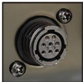
*Compatible machines feature a circular 8 pin connector.*
