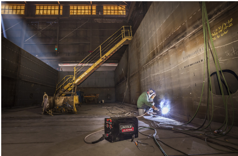
CrossLinc™ Technology provides voltage control at the point of use without a bulky and expensive control cable.
