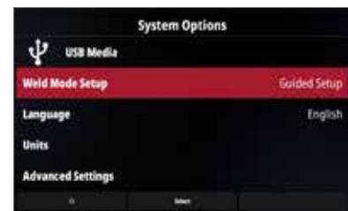
Following the indications on the screen, selecting the material type, thickness and type of joint the **Guide Setup** will set all correct parameters for an easy and qualitative weld
