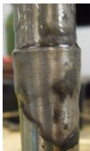
Black flux turns clear, (transparent), close to brazing application temperature. This is a useful indicator in timing braze wire application.
