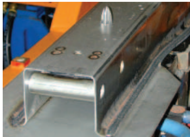
The Tandem MIG relies on Waveform Control to synchronize its dual arc system
