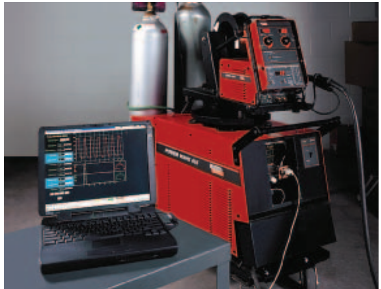
Alterations to the waveform can be made during the weld, using software created by Lincoln Electric.
