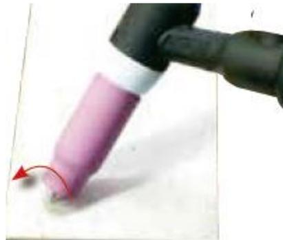
(14) With a small movement rotate the gas cup forward so that the tungsten electrode touches the work piece.
