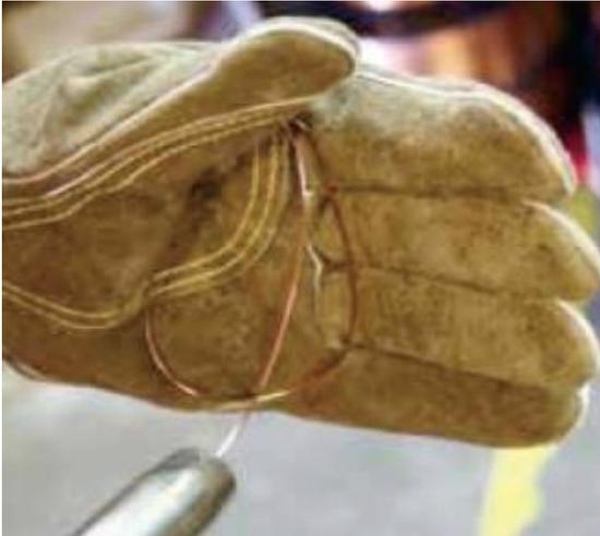
(8) A simple check for the correct drive tension is to bend the end of the wire over hold it about 100mm from your hand and let it run into your gloved hand, it should coil round in your hand without stopping and slipping at the drive rolls, increase the tension if it slips.
