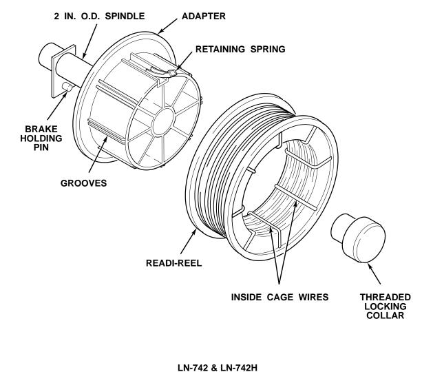
FIGURE B.5 - INSTALLING A 30 LB READI-REEL PACKAGE.
