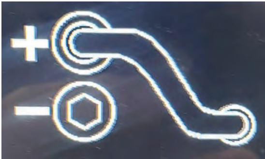
Figure B.3 Wire drive connected for positive polarity
