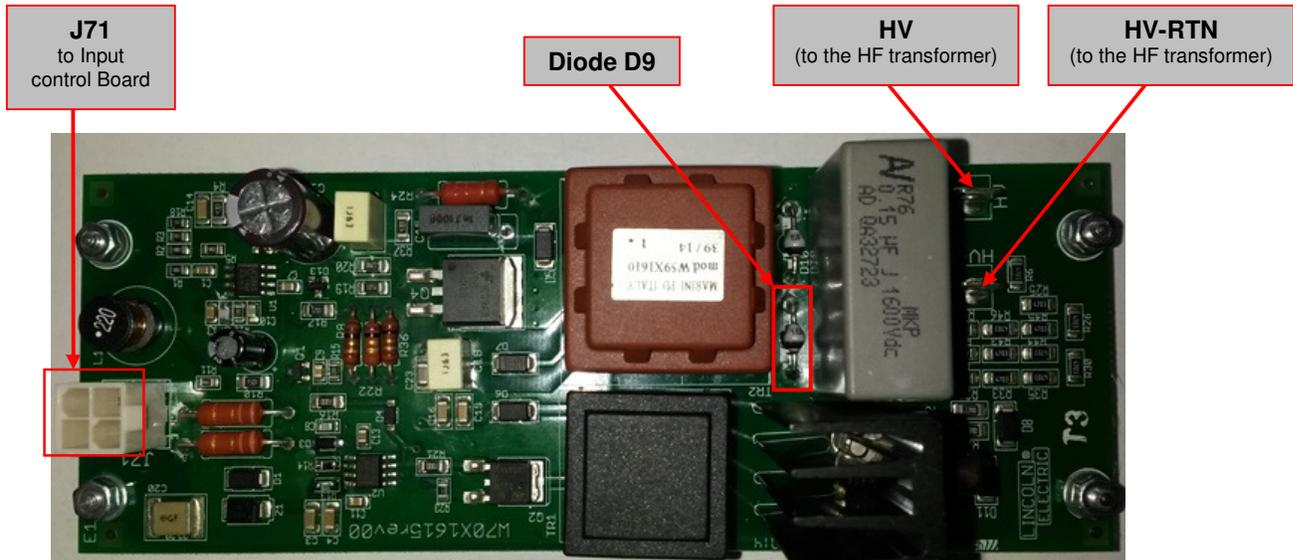
Figure 19 – W05X1615 HF board test points
