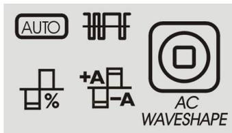
These icons allow the operator to customize the arc-performance for TIG welding in AC polarity only. AUTO and Expert Mode:
