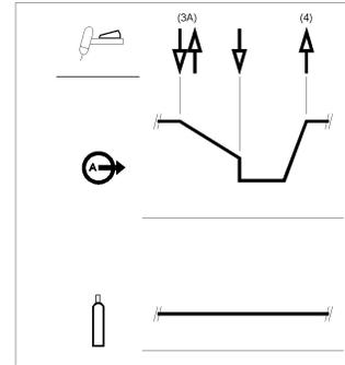
As shown here, again after the TIG torch trigger is quickly pressed and released from step 3A, it is possible to quickly press and release the TIG torch trigger a second time to end the downslope time and stop welding.
