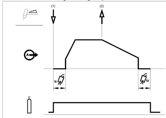
1. Press and hold the TIG torch trigger to start the sequence. The machine will open the gas valve to start the flow of the shielding gas. After the preflow time, to purge air from the torch hose, the output of the machine is turned ON. At this time the arc is started according to the selected welding mode. The initial current is set to 25A for LIFT starting (starting current parameter is disabled in the sequencer) or set according to the Starting current parameter for
