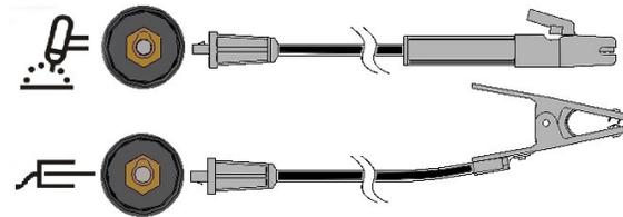
Connect the electrode cable to the torch terminal and the work clamp to the work piece terminal. Insert the connector with the key lining up with the keyway and rotate approximately ¼ turn clockwise. Do not over tighten.
