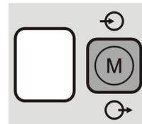
The memory function is designed to allow the operator to save up to 9 specific welding procedures. This memory button will have two functions:
