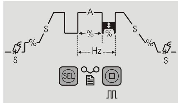
The sequencer allows for the customization of the TIG welding operation both in AC & DC- polarities. Pressing the "Sel" button will cycle through the process graph.
