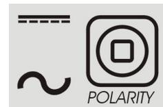
This icon is designated to set the polarity of the process in use: DC+, AC stick, DC- & AC TIG operations.
