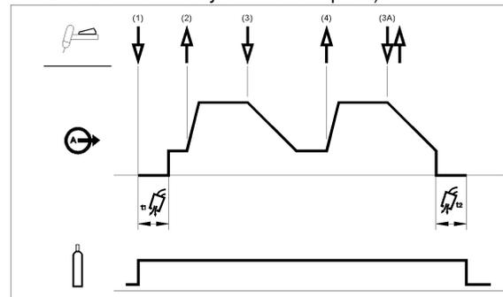
3. Press and hold the TIG torch trigger. The machine will now decrease the output current at a controlled rate, or downslope time, until the Crater current is reached.
