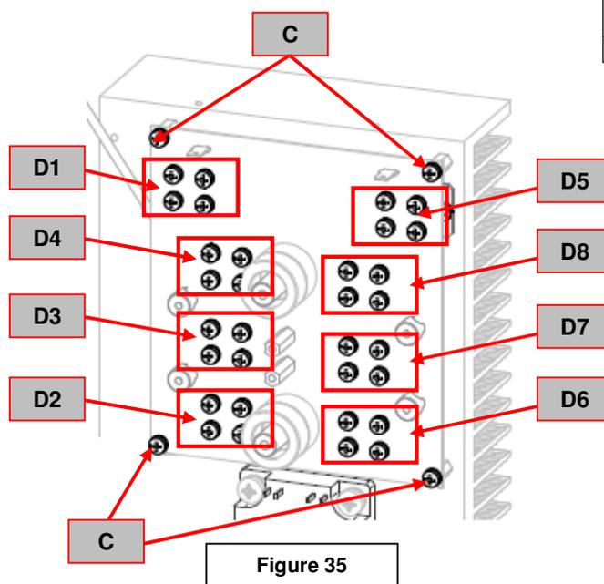
9. Using the Phillips screwdriver remove the 4 screws from each diode module **D1, D2, D3, D4, D5, D6, D7** and **D8**. Carefully remove the silicon sealant to access the screws if present. See **Figure 35**
