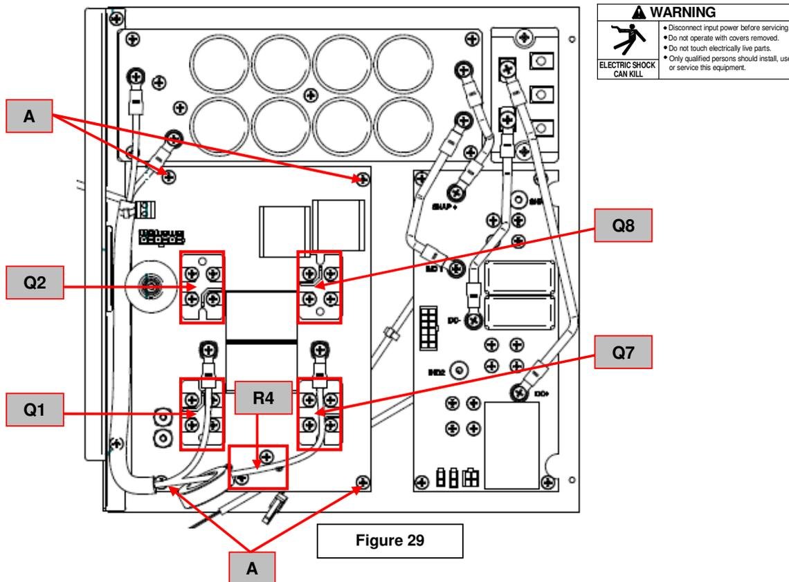
10. Using the Phillips screwdriver remove the 4 screws from each module **Q1**, **Q2**, **Q7** and **Q8**. Carefully remove the silicon sealant to access the screws if present. See **Figure 29**
