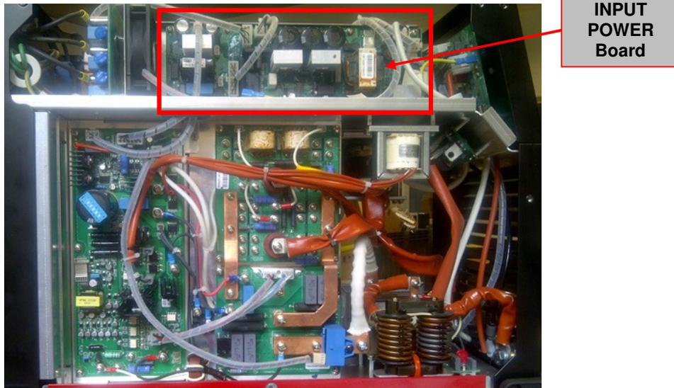
Figure 6 – W05X1461 INPUT POWER Board location
