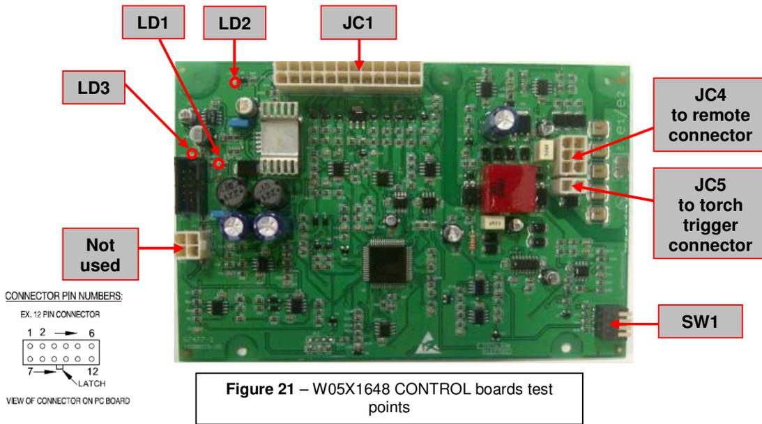
Figure 21 – W05X1648 CONTROL boards test points
