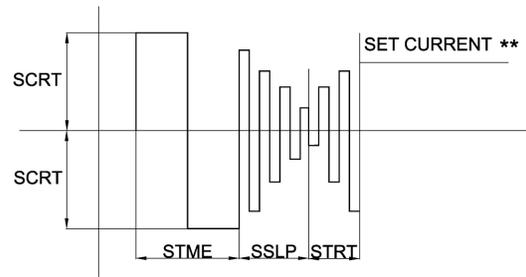
The starting sequence changes also if the foot paddle is present: in fact taking care of the STRT level is not settable, the level at the end of the SSLP ramp is the level from the footpaddle or the PCRT level.
