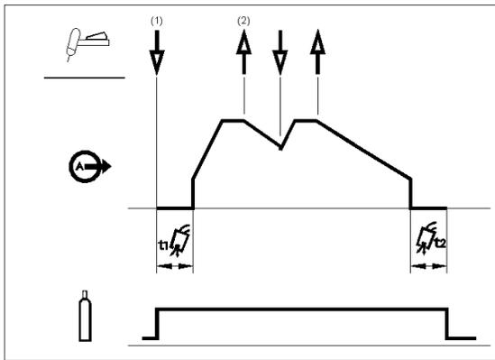
1. Press and hold the TIG torch trigger to start the sequence as described above.
