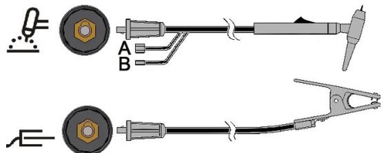
Connect the torch cable to the torch terminal of the machine and the work clamp to the work piece terminal. Insert the connector with the key lining up with the
