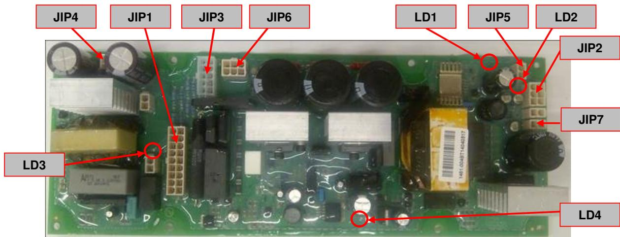
Figure 7 – W05X1461 INPUT POWER Board Test Points
