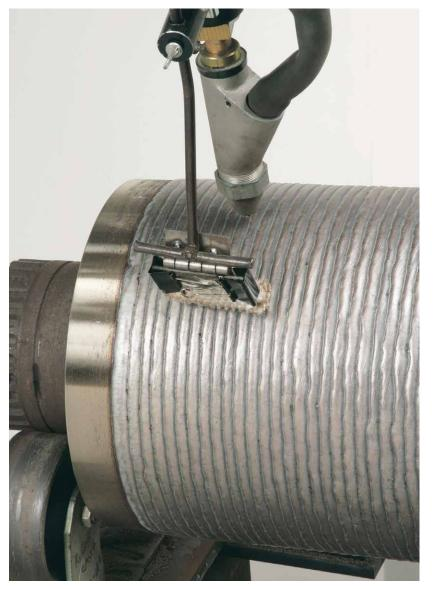
A faster, smaller bead tends to freeze quicker than a slow bead.
