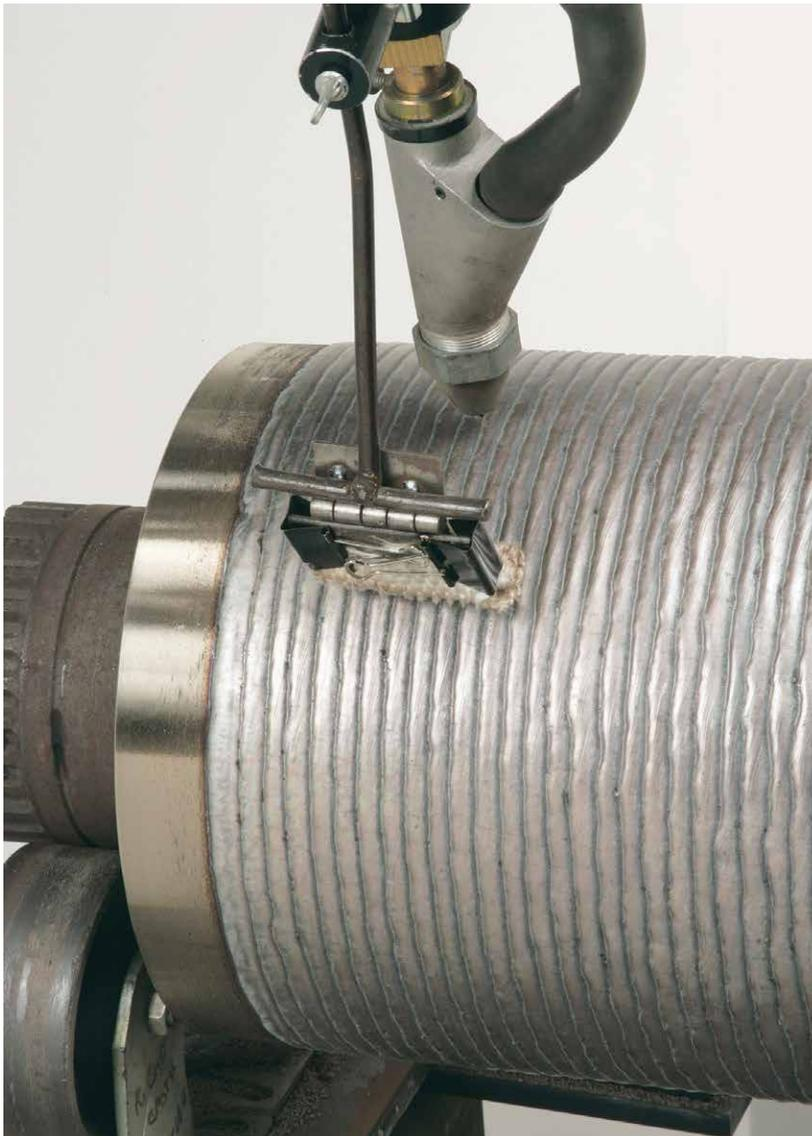
A faster, smaller bead tends to freeze quicker than a slow bead.
