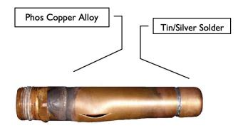
Note the distortion next to the brazed connection in the picture. Higher temperature brazed connections always fail adjacent to the braze. This failure occurs at a much lower pressure than those connections soldered with a tin/silver alloy. This makes tin/silver a better option than higher temperature phos/copper/silver braze alloys.
