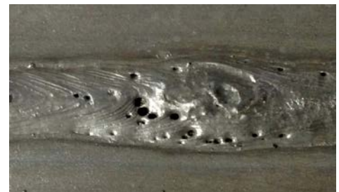
Figure 9-7: Gas Pockets in the Weld Resulting from Insufficient Flux Coverage
