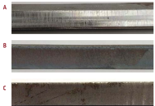
Figure 9-4: Good Porosity-Free Welds Can Be Made on Machined and Flame-Cut Edges and on Uncut Edges that Have an Ordinary Amount of Mill Scale. See A, Machined Edges; B, Flame-Cut Edges; C, Uncut Edges.
