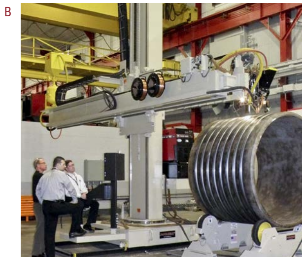
Figure 2-16: A, Robotic SAW; B, Hard Automation
