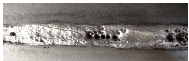
Figure 9-6: Porosity Caused by Oily Plates.
