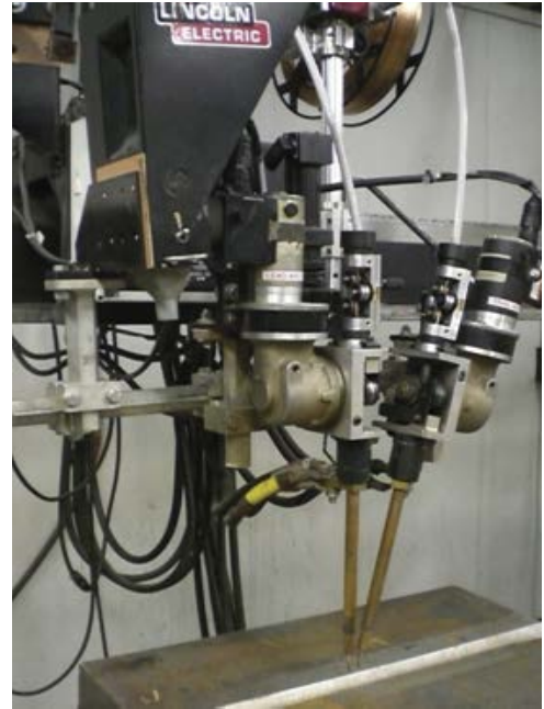
Figure 6-2: DC-AC Double Electrode Tandem Arc Setup
