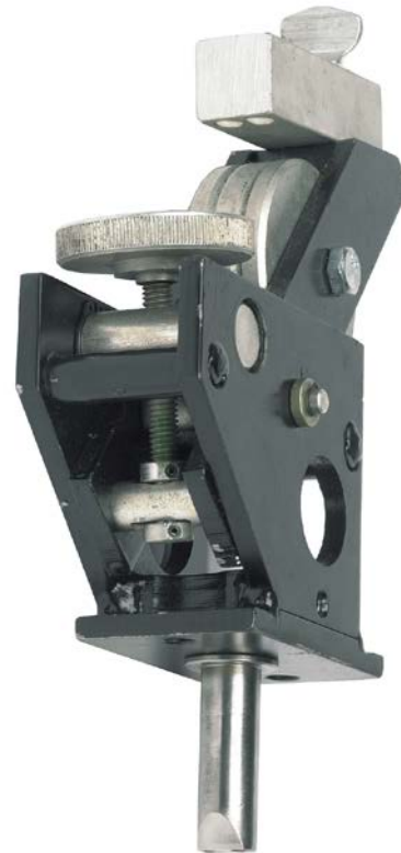
Figure 7-10: The Lincoln Electric Tiny Twinarc Solid Wire Straightener Accommodates Wire Diameters 0.045 in. – 3/32 in. (1.2 through 2.4 mm). It Is Particularly Valuable on Longer CTWD Procedures.
