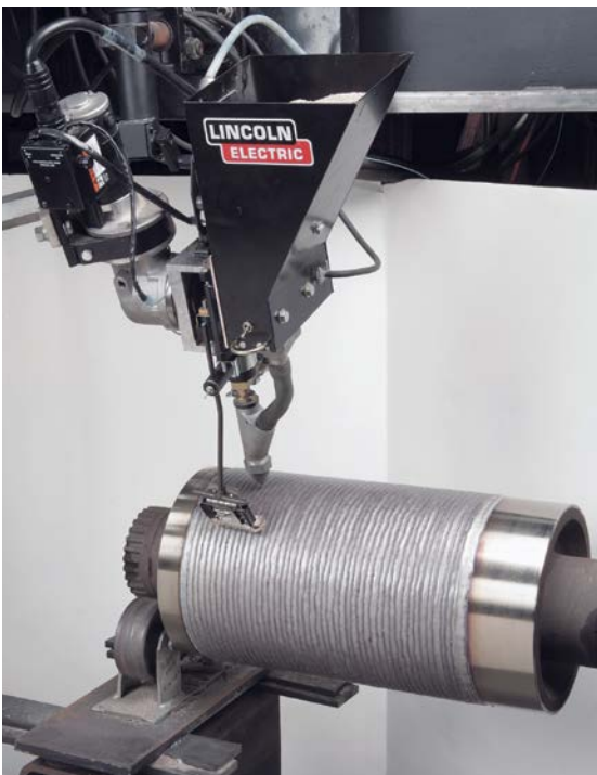
Figure 8-3: Caster Roll Rebuilding Using Hardfacing SAW
