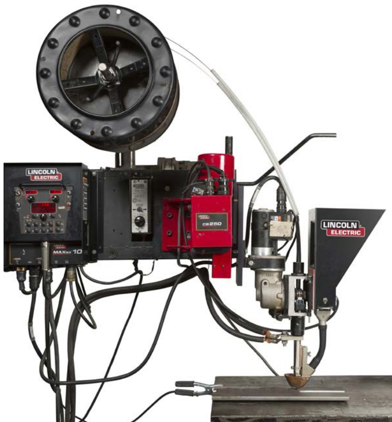
Figure 2-18: A Tiny Twinarc® Welding Cell
