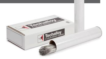
**Tech-Rod**® **309/309L** electrodes have reduced carbon levels (0.04% max) that offers increased resistance to inter-granular corrosion. Type 309/309L is ideal for joining stainless steels to themselves or to carbon or low alloy steels, and can be used at temperatures of up to 700°F (371°C). Reduced carbon levels help prevent intergranular corrosion.
