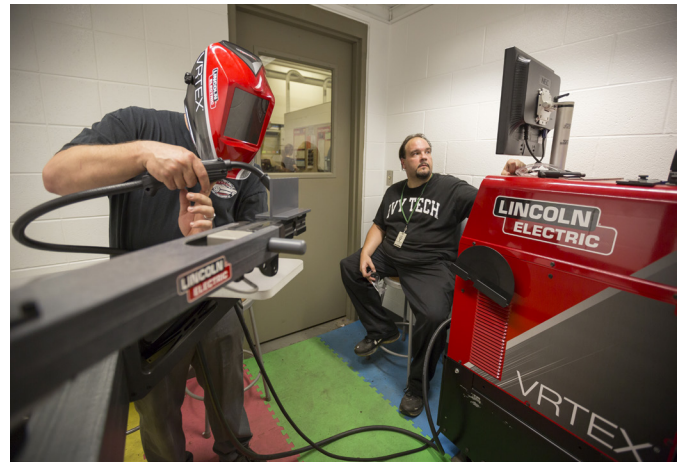
Every student begins the Weld 101 class with up to two weeks on the VRTEX 360 virtual reality welding simulator to practice position, angles and travel speed without burning plate, rod, wire or shielding gas.
