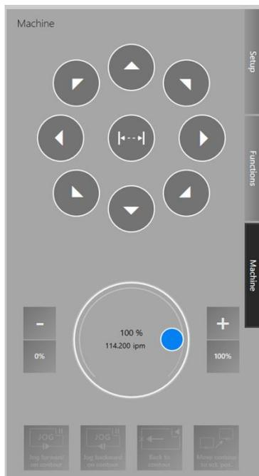
Select and hold a **Direction Arrow** on the jog pad to move the cutting head in that (X/Y) direction. Release to stop moving.
