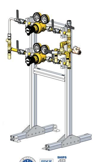
The Model 1030 is a high flow gas supply manifold intended to be attached downstream of a bulk gas system/vaporizer and which will regulate the pressure and flow of gas into facility pipelines. The manifold utilizes the Harris Model 3550-250 regulators with stainless steel diaphragms. Flow rates up to 10,000 scfh can be achieved at the nominal inlet pressure of 350 psi. The system has a 450 psi maximum rated inlet pressure.
