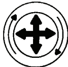
Rotate the filter while pulling straight out.
