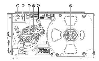
Figure 3: Wire Compartment
