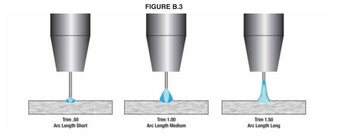
Most pulse welding programs are synergic. As the wire feed speed is adjusted, the POWER WAVE® S500CE will automatically recalculate the waveform parameters to maintain similar arc properties.
