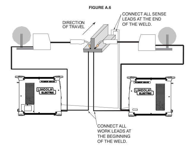
• For circumferential applications, connect all work leads on one side of the weld joint, and all of the work voltage sense leads on the opposite side, such that they are out of the current path.
