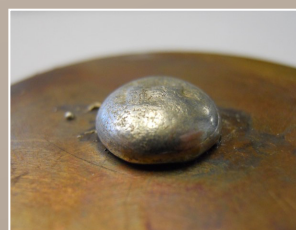
Fig. 5 Solder nonwetting without flux
