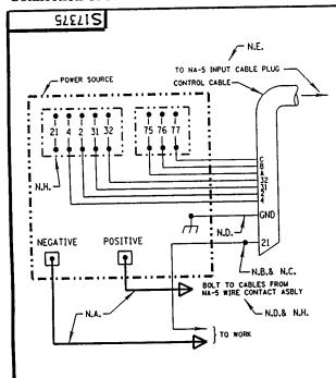
Above diagram shows electrode connected positive. To change polarity, turn power off, reverse the electrode and work leads at the power source and position the switch on power source if equipped, to proper polarity. Refer to NA-5 Deparating Manual for required NA-5 control box polarity connections. Also refer to note N.H.
