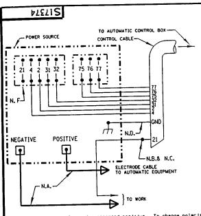
Above diagram shows electrode connected positive. To change polarity, turn power off, reverse the electrode and work leads at the power source and position the switch on power source (if equipped) to proper polarity. Reverse the leads on the back of the ammeter and voltmeter in the automatic control box. Also refer to note N.F.
