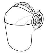
**Step 2 -** After the adjustment knobs, remove the o-rings and washers from each side.
