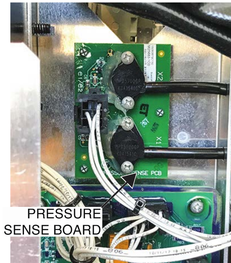
Figure F.51 – Pressure sense board plug J4 location
