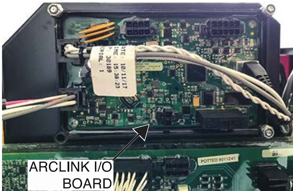
Figure F.48 – Arclink I/O board plug and LED locations
