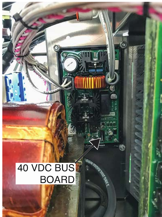
Figure F.53 – 40 VDC bus board location
