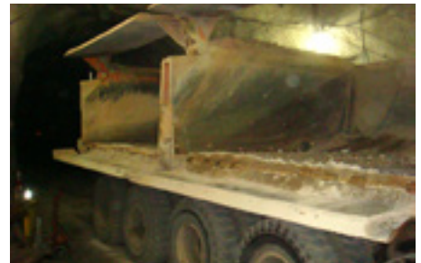
Weartech wear plates remain in service after hauling over 3 million tons in 28 months
