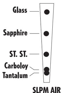
Floats made from more dense materials will rise less thereby yielding higher flow capacities. Relative flow capacities for some common float materials are shown above.
