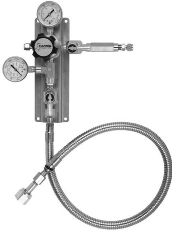
Model SG 770 provides a continuous backup supply of gas in case of generator failure or loss of power. The system automatically switches to a backup cylinder of gas when the generator supply pressure drops below a preset value. The process will automatically reverse when the gas supplied by the generator returns to a normal level. All units include the following:
