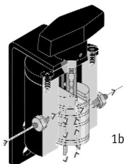
Figures 1a and 1b. The "plus" valve (a) features a closed gas path when changing cartridges. When placed in the down position (b), the "plus" valve shifts gas through the cartridge.
