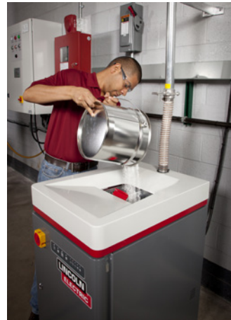
Shown: Limestone powder being added to an Oil Guardian™
