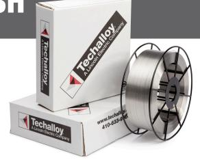
**Techalloy**® **308/308H** electrodes are used to weld unstabilized austenitic stainless steels such as 302, 304H and 305. Techalloy® 308/308H electrodes provide a high carbon deposit (minimum of .04% carbon) for high temperature applications. Typical applications include chemical, petrochemical industries as well as distillery, dairy and restaurant equipment.
