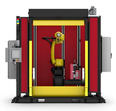
Render is for reference only and shows the following options: Single Robot Configuration, Headstock/Tailstock Positioner, HMI Control Panel, High Voltage Power Distribution Panel, Power REAM® Torch Maintenance Station
