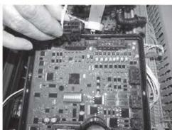
7. Reconnect the input power and assure proper output.
