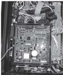
6. 6- Reconnect the J331 connector to J88 on the S30221-[ ] (G6752-[ ]) board, then reconnect the rest of the connectors.
