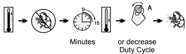
The machine is protected from overheating by a temperature sensor.
