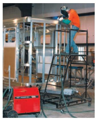
The Power MIG 300 is operated with one-knob synergic control, allowing users to set parameters such as wire feed speed. The unit will automatically adjust itself to the corresponding proper voltage and will constantly monitor the changing characteristic of the arc, making the unit easy to use, even for the novice welder.
