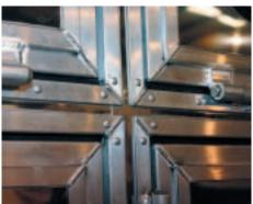
nature of the welding at Dream Coach Trailer Company—thin aluminum, all-position work and tight space requirements. In addition, imperfections in the polished aluminum composing these trailers cannot be easily masked. Attaining attractive weld bead appearance is critical
