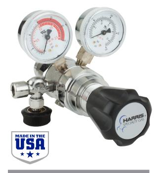
Model HP 717 is a uniquely designed regulator for acetylene applications. This regulator prevents overdrawing the acetylene cylinder where acetone or other solvents can be pulled into the gas stream and damage downstream equipment. The regulator shuts off the flow of gas when acetylene cylinder pressures become too low to support the process. Outlet needle valve for flow control comes with all units.
