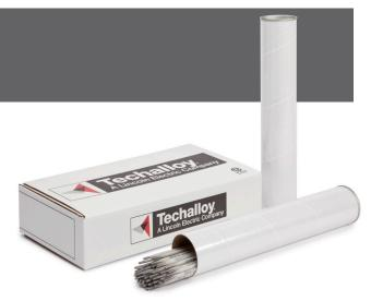
Tech-Rod<sup>®</sup> 630 is a precipitation hardening stainless steel covered electrode used for welding materials of similar chemical composition such as 17-4 and 17-7. Can be used in the as welded condition or may be heat treated to obtain higher strength. Mechanical properties of the alloy are greatly influenced by the heat treatment.
