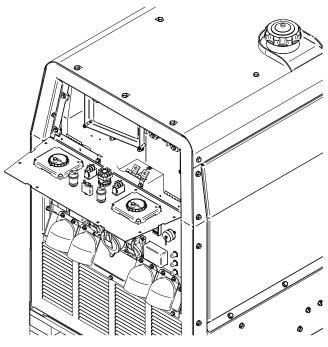
Locate VRD switches (as marked in Fig A.2) on both PC control boards. Left position on each switch indicates "OFF" state; right position on each switch indicates "ON" state. PC Control Board on the left is for settings for the left user. PC Control board on the right is for settings for the right user.
