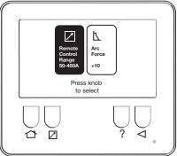
All weld modes support using a remote control like K857-1. Plug the remote into the 6 pin connector on the front of the machine.
