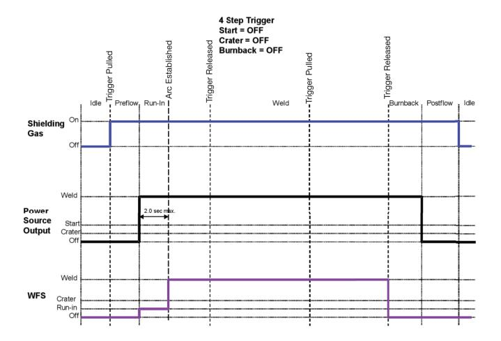
Example 2: 4-Step Trigger: Manual Control of Start and Crater times with Burnback ON.
