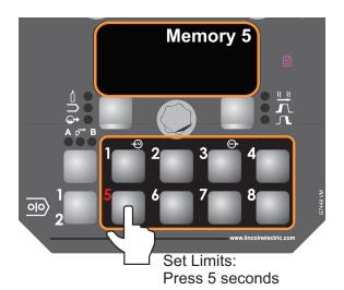
If the passcode does not equal zero (0000), enter the passcode now. If the passcode has been forgotten, a computer application is required to change the passcode.
