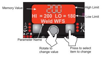
The Limits Setup menu shows a list of all parameters available for the weld mode stored in the memory chosen. For example, if limits are being set for a stick (SMAW) mode, parameters such as Run-in WFS and Postflow will not appear.
