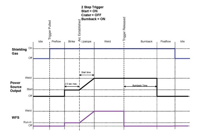
Example 3: 2-Step Trigger: Customized Arc Start, Crater and Arc End
