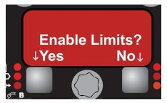
Press the left button (YES) to enable limits or the right button (NO) to disable limits. Disabling limits does not change any limits values that may have been previously set.
