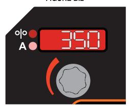
The left display and knob are used to adjust either wire feed speed or amperage, depending upon the process selected.
