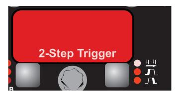
2-Step Trigger controls the welding sequence in direct response to the trigger. When the gun trigger is pulled, the welding system (power source and wire feeder) cycles through the arc starting sequence and into the main welding parameters. The welding system will continue to weld as long as the gun trigger is activated. Once the trigger is released, the welding system cycles through the arc ending steps.
