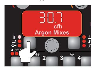
To display the actual gas flow, press the left button to select the shielding gas LED and then press the gas purge button. To display gas flow while welding, change P.3 in the set-up menu to "Show Gas Flow Rate."
