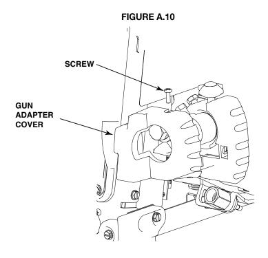
3. With a 3/4" wrench, remove the bolt holding the electrode lead to the gun adapter.
