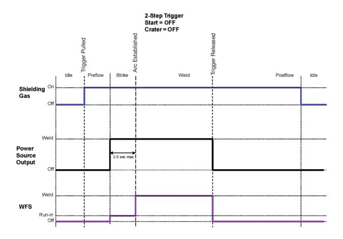
Example 2: 2-Step Trigger: Improved Arc Start and Arc End
