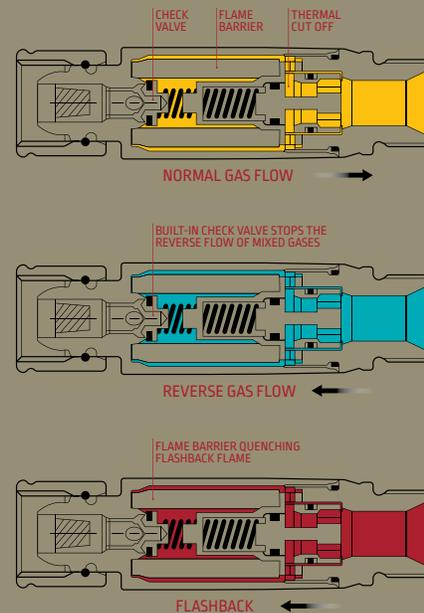
Exercise caution when selecting the proper FBA capacity or adding additional FBAs to gas lines. All FBAs are restrictive. Compensating for restrictions should be done before lighting. Improper selection or use can make conditions worse than not having any FBA protection at all.
