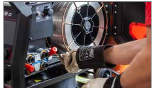
Full access for wire spool installation
