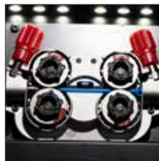
Professional wire feeding system features four driven wire feed rolls. Excellent wire feeding on every material. Permanent internal lights makes changing easier.
