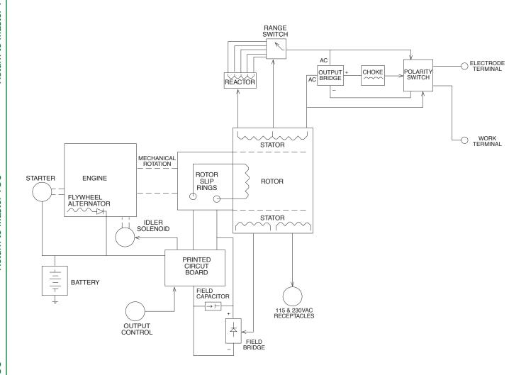
FIGURE E.1 - RANGER 8 BLOCK LOGIC DIAGRAM
