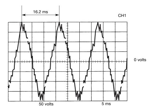
This is the typical AC output voltage generated from a properly operating machine. Note that each vertical division represents 50 volts and that each horizontal division represents 5 milliseconds in time.
