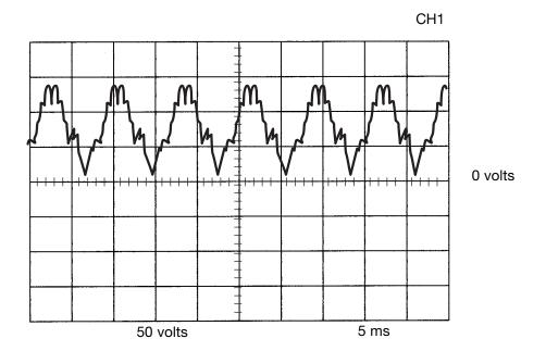
This is the typical DC output voltage generated from a properly operating machine. Note that each vertical division represents 50 volts and that each horizontal division represents 5 milliseconds in time.
