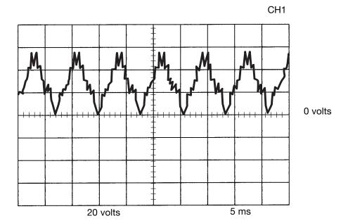
This is the typical CV output voltage generated from a properly operating machine. Note that each vertical division represents 20 volts and that each horizontal division represents 5 milliseconds in time.
