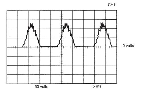
This is NOT the typical DC (+) output voltage waveform. One output diode is not functioning. Note the "gap" in the waveform. One output diode was disconnected to simulate an open or nonfunctioning output diode. Each vertical division represents 50 volts and each horizontal division represents 5 milliseconds in time.
