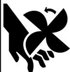
1.d. Keep all equipment safety guards, covers and devices in position and in good repair. Keep hands, hair, clothing and tools away from V-belts, gears, fans and all other moving parts when starting, operating or repairing equipment.
