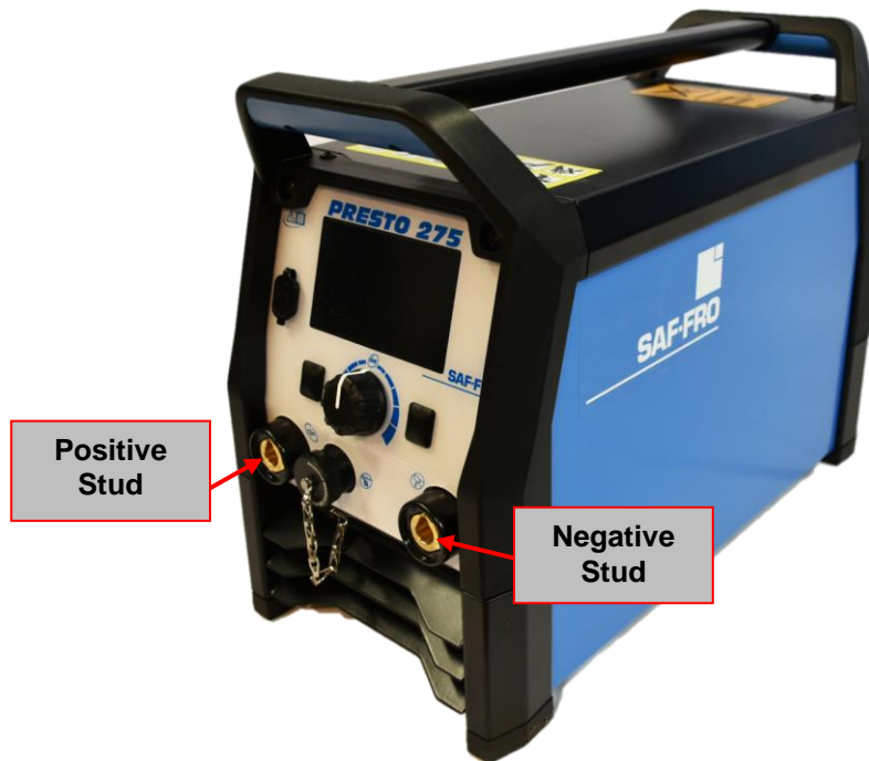
Figure 8 – Output studs location
