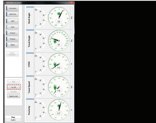
When ready, simply pull the trigger. The program will start recording data. The trainee can now start moving along the joint. Make sure the gages are not red prior to or during Arc Off welding. If the trainee is leaning over the torch and happens to cover the target, the gages will turn red and data will not be saved.
