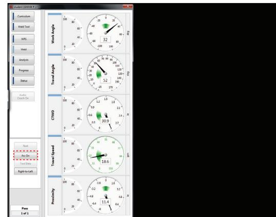
In Arc On mode, 'Start' and 'Stop' icons are disabled. When the trainee is ready to weld, they can just start welding. The program will automatically start recording data once an arc is struck and it will save that data once stopped. Make sure the gages are not red prior to or during Arc On welding. If the trainee is leaning over the torch and happens to cover the target, the gages will turn red and data will not be saved.
