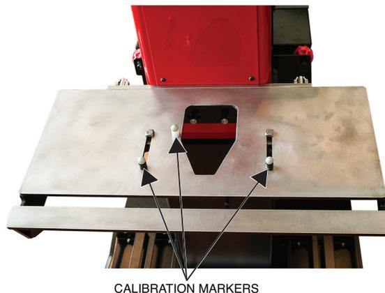
7. With the LED markers in place, select the 'Start Calibration' icon on the screen. The LED markers on the screen will start to blink while various numbers appear above them. During this time, the equipment is determining the position of the fixture platform. See Figure B.40.
