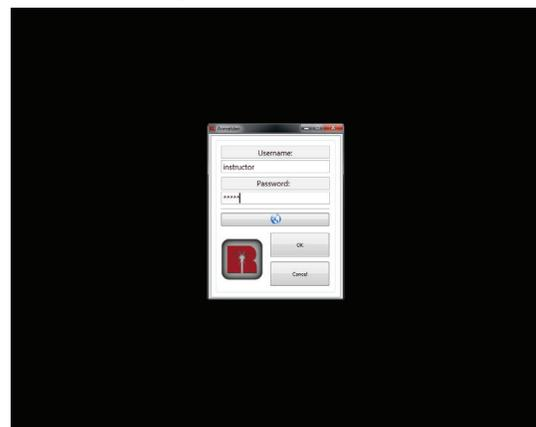
3. Using the touchscreen monitor, select the 'OK' icon on the login window. Once selected, the user will be logged in and a set of menu options, specifically for an instructor, will be displayed on the left side of the screen. See Figure B.8.
