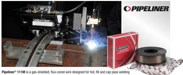
of X80 to X100 grade pipe. Optimized for automated and semi-automatic pipe welding applications, Pipeliner® 111M has a consistent arc and fast freezing slag to maintain a flat bead shape all around the pipe. The electrode is capable of producing Charpy V-Notch impact properties exceeding 27 J (20 ft•lbf) @ -40°C (-40°F). For an electrode that meets the demands of automated and semi-automatic pipe welding on up to X100 grade pipe — choose Pipeliner® 111M.
