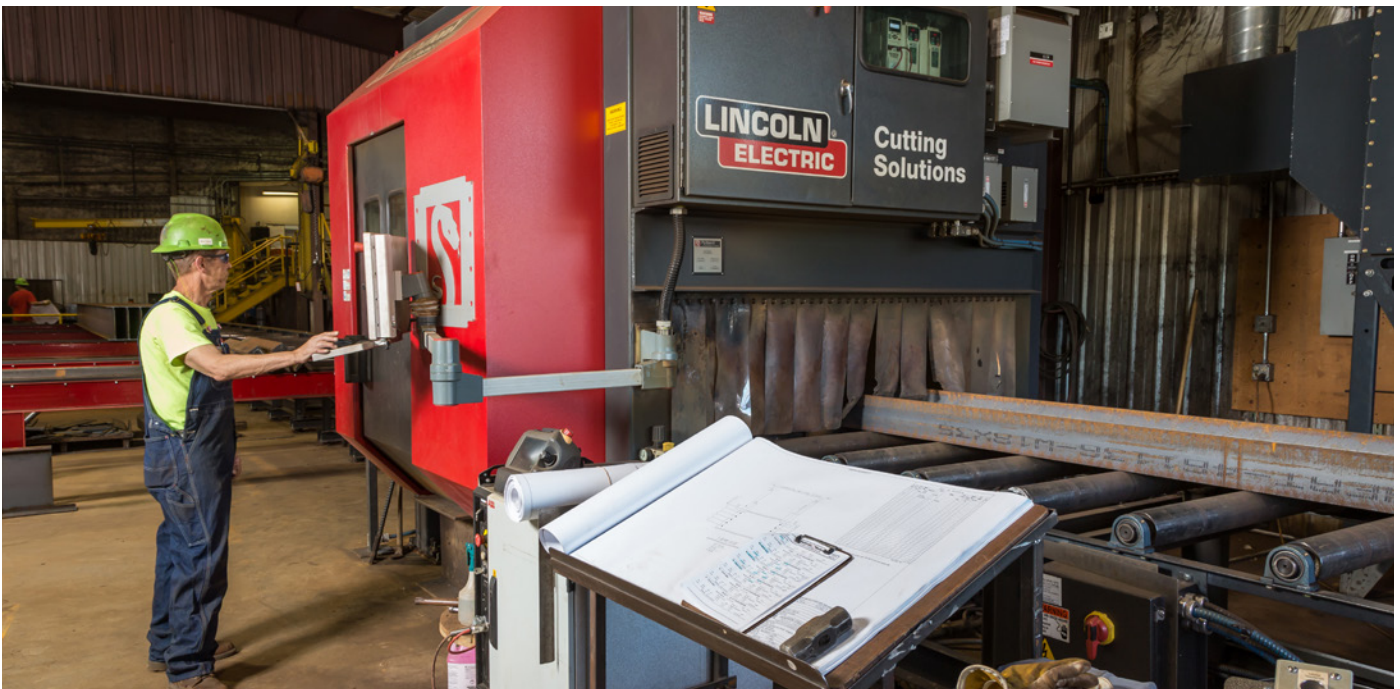
Operator programming the PythonX for beam production
