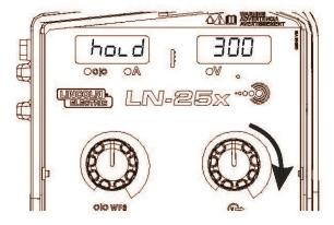
Press the set-up button to exit the set-up menu.
