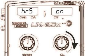
Press the set-up button to enter the hold display menu.
