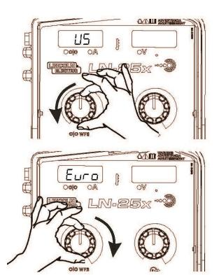
Press the set-up button again to enter the Run-In menu.
