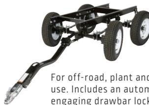
For off-road, plant and yard use. Includes an automatically engaging drawbar lock when the drawbar is raised to the vertical position.
