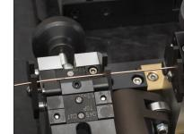
2 Remove the flash in the wire joint using the Wire Sizer.
