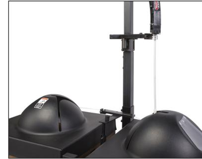
**4** When wire from box 1 runs out, the transfer arm will switch over to box 2. Simply replace empty box and repeat steps 1-3.
