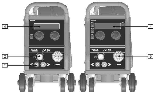
1. Water Connectors: Connections for water cooled torches.
